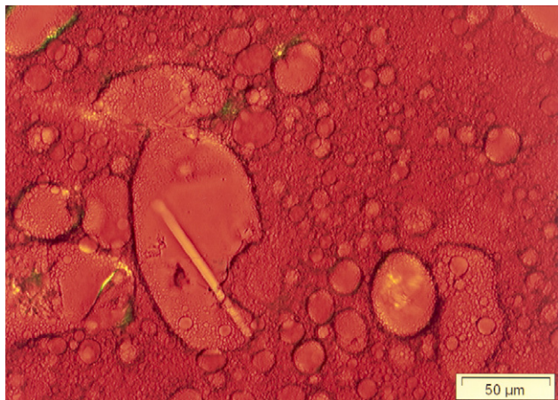
Fig. 6. Emulsion stressed at shear rate \dot{\gamma} = 1000 \text{ s}^{-1} and duration t = 100 \text{ s} (strain units = 1000 \text{ s}^{-1} \times 100 \text{ s} = 100,000 at 40^\circ\text{C} ).
